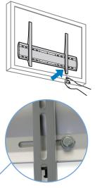
Security fasteners on mounting brackets prevent easy removal of the display
