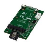
The SAT32MSATM SATA to mSATA adapter enables you to connect an mSATA SSD to any standard SATA port, ideal for connecting an mSATA SSD to an ITX computer systems that does not have an mSATA port.
