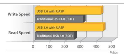
At the same peak in testing UASP also shows an 80% reduction in required processor resources.
