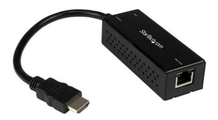
This compact transmitter uses HDBaseT<sup>™</sup> technology to extend your HDMI® signal up to 230 feet (70 meters) over a single CAT5e or CAT6 cable, to an HDBaseT display, projector or receiver (sold separately). The transmitter supports Ultra HD and Full HD video resolutions (4K and 1080p), with support for the accompanying digital 7.1 audio.
