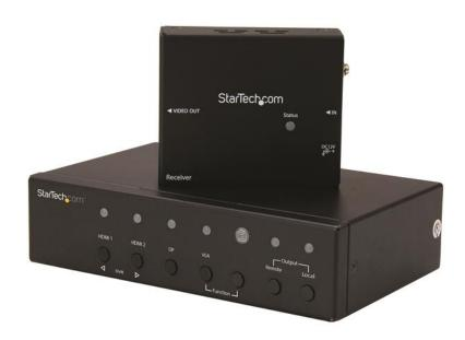
This multi-input video extender kit uses HDBaseT $^{\text{TM}}$  technology to extend your video signals up to 230 feet (70 meters) over a single CAT5e or CAT6 cable. It features a built-in video switch that enables you to choose which video source is outputted from four independent video sources (2 x HDMI, 1 x VGA and 1 x DisplayPort). The video extender supports Ultra HD 4K and Full HD 1080p video resolutions, with support for the accompanying digital 7.1 audio.
