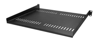
This 1U rack shelf lets you add 16 in. of flat storage space to any EIA-310 compliant server rack or cabinet. The shelf is vented to improve air flow and help lower temperatures in your rack.
