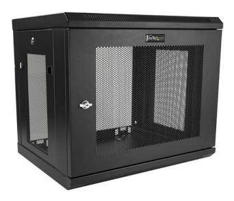
This 9U server rack cabinet lets you mount your EIA-310 compliant equipment to the wall. The enclosure features an adjustable mounting depth from 6 to 17 in. and offers a maximum load capacity of 200 lb. (90 kg).
